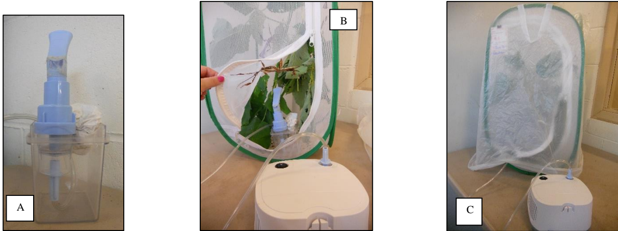
Figure 8. The F10 SC Veterinary Disinfectant nebulizer set up. A) The F10 solution is placed in the bottom portion of the nozzle and is secured upright in a magenta with a paper towel. B) The magenta is placed inside the pop-up caterpillar castle and a rubber hose is connected to the nebulizer. C) A clear plastic garbage bag is placed over the top to hold in the medicated mist.
