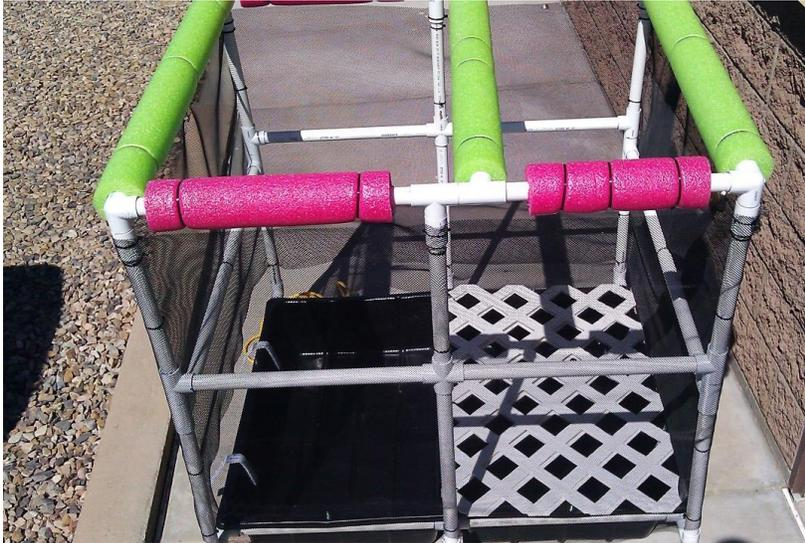
The "Floater Float" is designed to suspend a California mussel groups beneath the surface of the lake where the water temperature is cooler.
