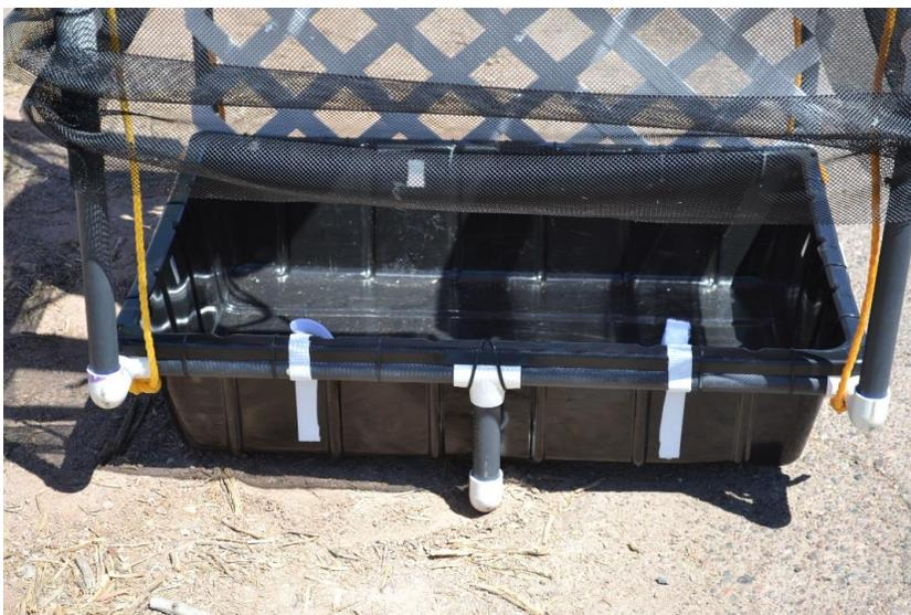
The tub consists of a 36" x 30" x 8" inch deep hard plastic. It is filled to a 5-inch depth with finely sifted silt.
